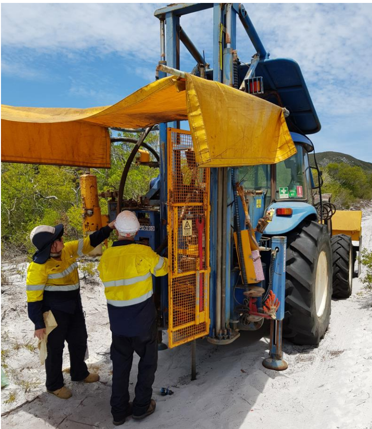
Yearlong Contracting Vacuum Drill rig
