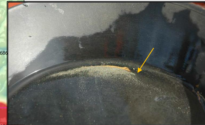
Fine gold produced after processing a sample with a petrol-powered mill. Source: Fairstar Resources (5)
