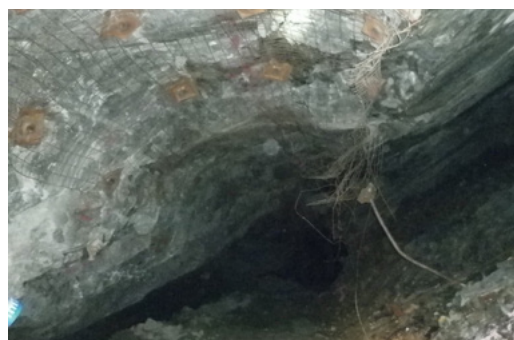
Above: Mined area from Citigold's test mining showing the floor of the level drive, and the stope voids (ore extracted area) above and below the level. The ore has been cleanly extracted, showing how the mining method minimizes dilution by maintaining a narrow stope 'slot' width.
