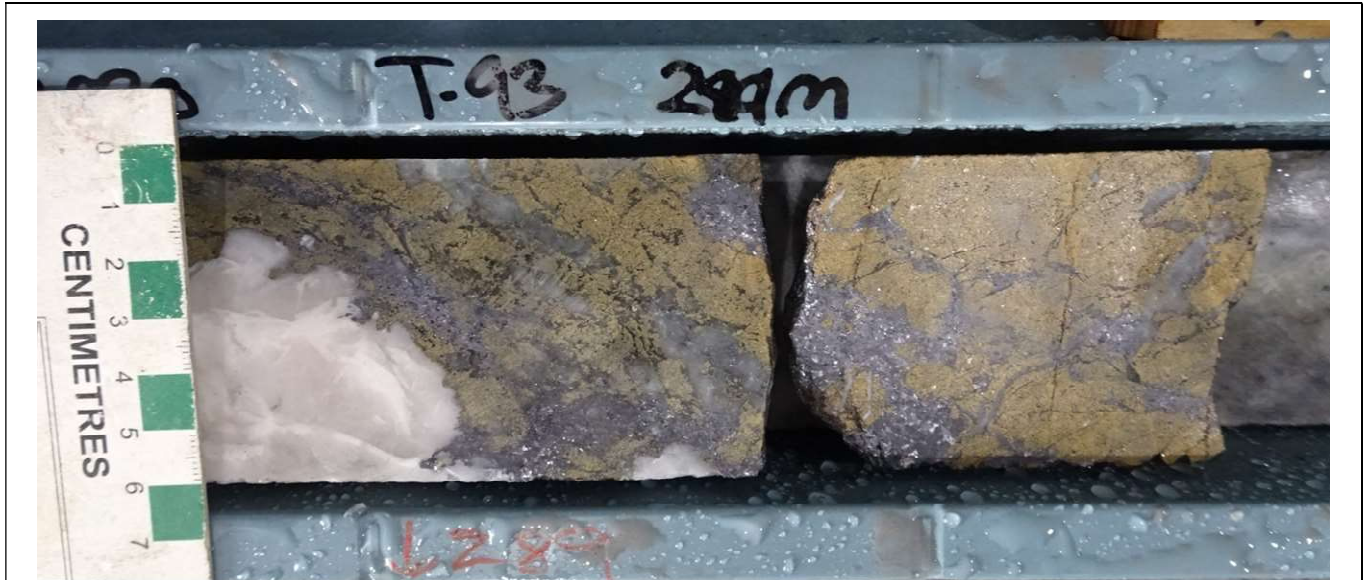
Photo 1 – Cullarin Gold Project - Hume Target – Drillhole HUD020 – 287.5m – massive sphalerite & galena.
