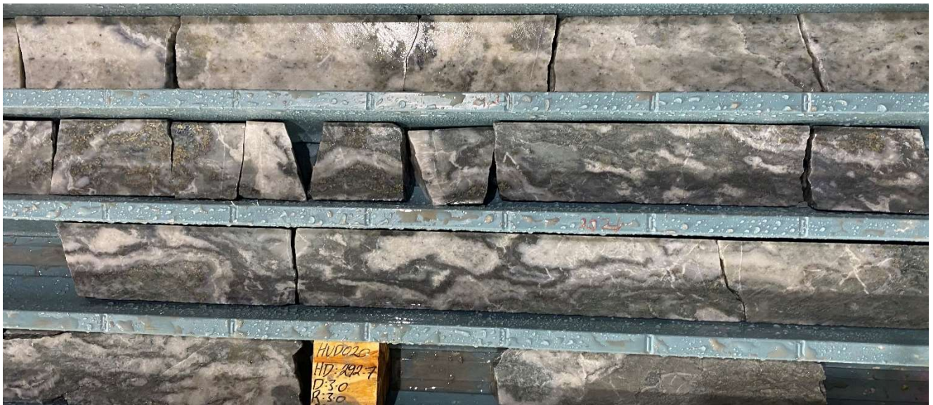
Photo 2 – Cullarin Gold Project - Hume Target – Drillhole HUD020 – 290-293.5m – intense, banded quartz-carbonate-veining with sphalerite & galena.
