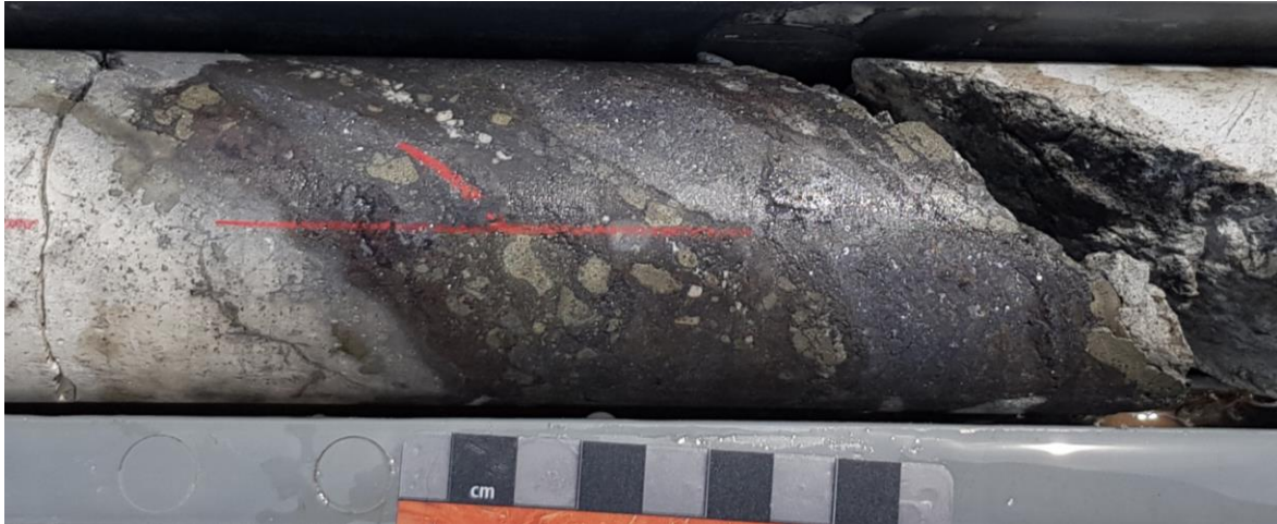
Figure 3. Sheeted high-grade vein pearcite, sphalerite, galena with brecciated pyrite blebs at 128.1m.
