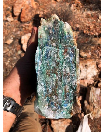
Figure 6: Rock chip MFN02 (212475E 6767617N MGAz51) which assayed 2% Cu, 2 g/t Au and 5.6 g/t Ag.
