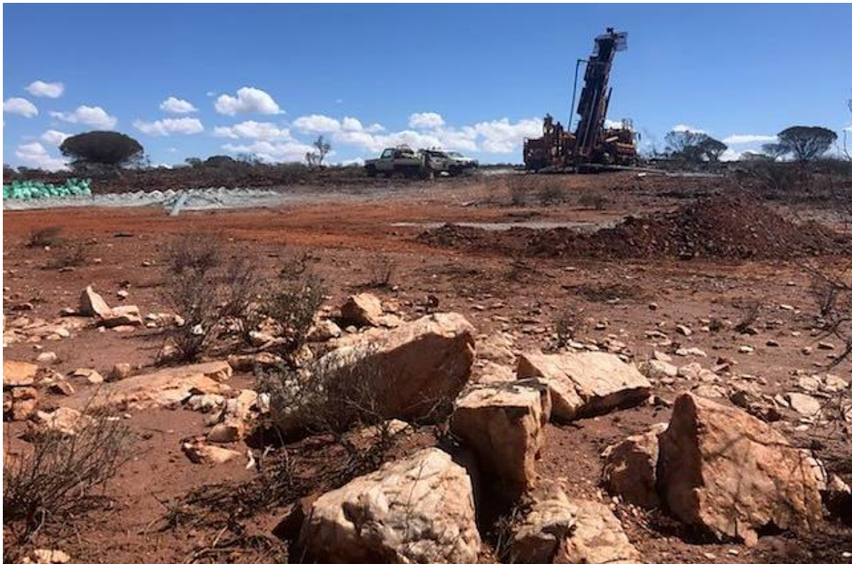
Figure 1: RC drill rig at Bald Hill with a subcropping Cu-Au-Ag vein in the foreground.
