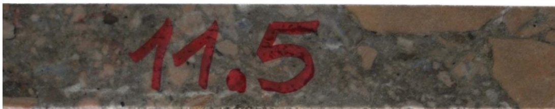
Figure 4: Examples of the mineralised core intercepted proximal to NE-SW trending fault in Area D, exhibiting intensely altered and brecciated calcareous sediments.
