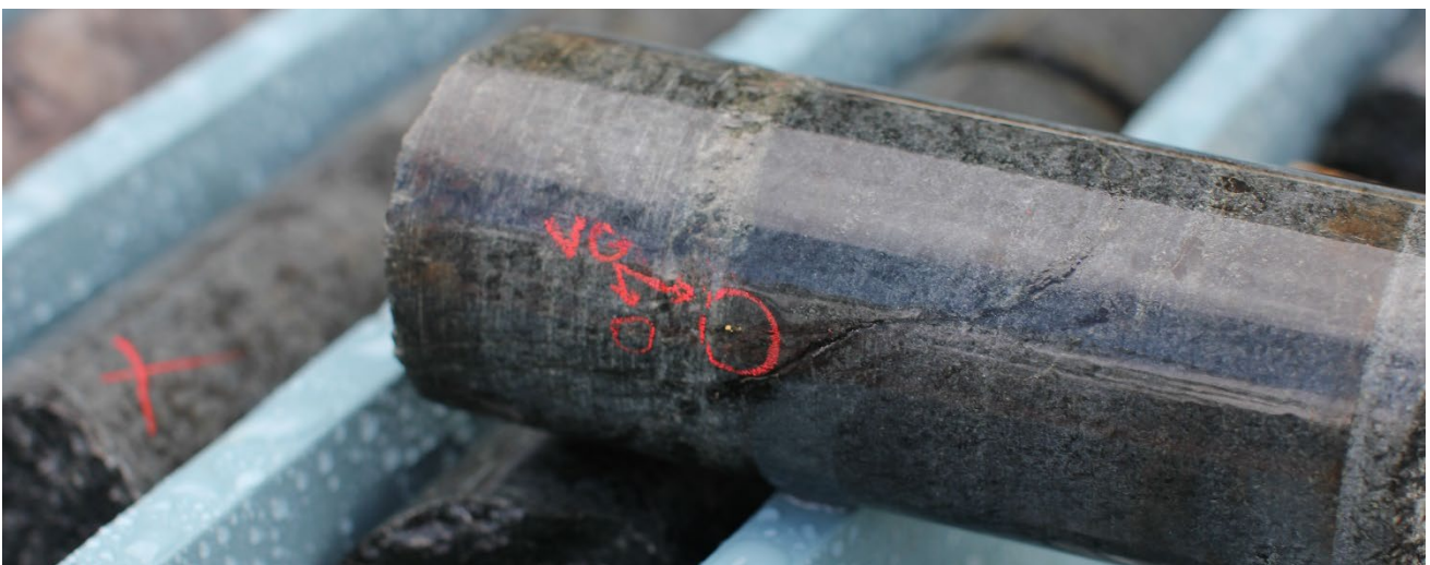
Figure 1 - Visible gold occurrence in RBDD005 drill-core (NQ), at 192.5m. Visible gold does not characterise all mineralised intercepts at Redback. The former owner reported visible gold was encountered in several drill-holes. These have been validated both by observation of remaining core and core photos.
