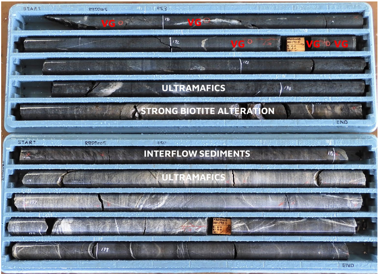
Figure 2 – Multiple visible gold occurrences highlighted in red circles in RBDD005 drill-core (NQ), from 190.85m to 192.5m. The visible gold is proximal to strong biotite alteration, adjacent to interflow sediments within the ultramafics, analogous to observations within the Wattle Dam Gold Mine.
