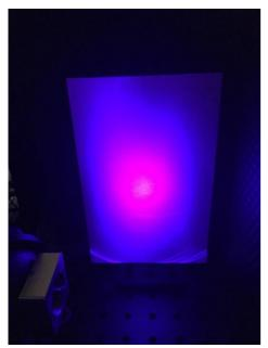
RPCVD is a low-temperature, ammonia-free approach to GaN-based epitaxial growth, with advantages not possible with conventional metal-organic chemical vapour deposition (MOCVD).
