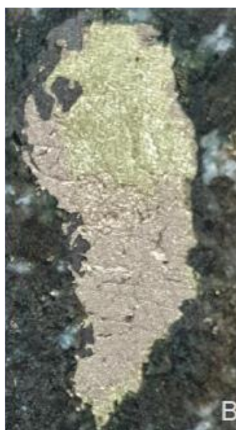
Figure 1A: A cut slab through rock chip GLRK008 showing multiple three-phase blebby magmatic sulphides within the Money Intrusion.
