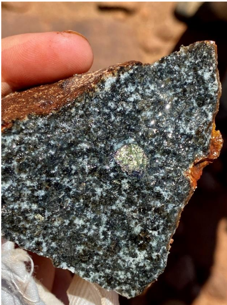
Figure 3: GLRK008A showing a three-phase blebby sulphide with chalcopyrite-pyrrhotite- pentlandite within a gabbro.
