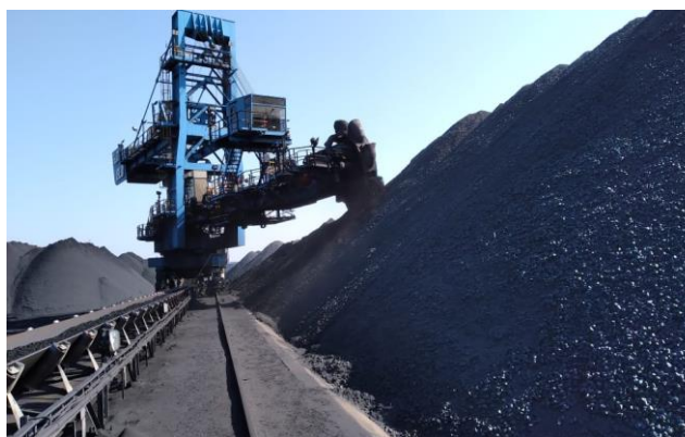
Image: reclaimer taking coal for loading on the ship.
