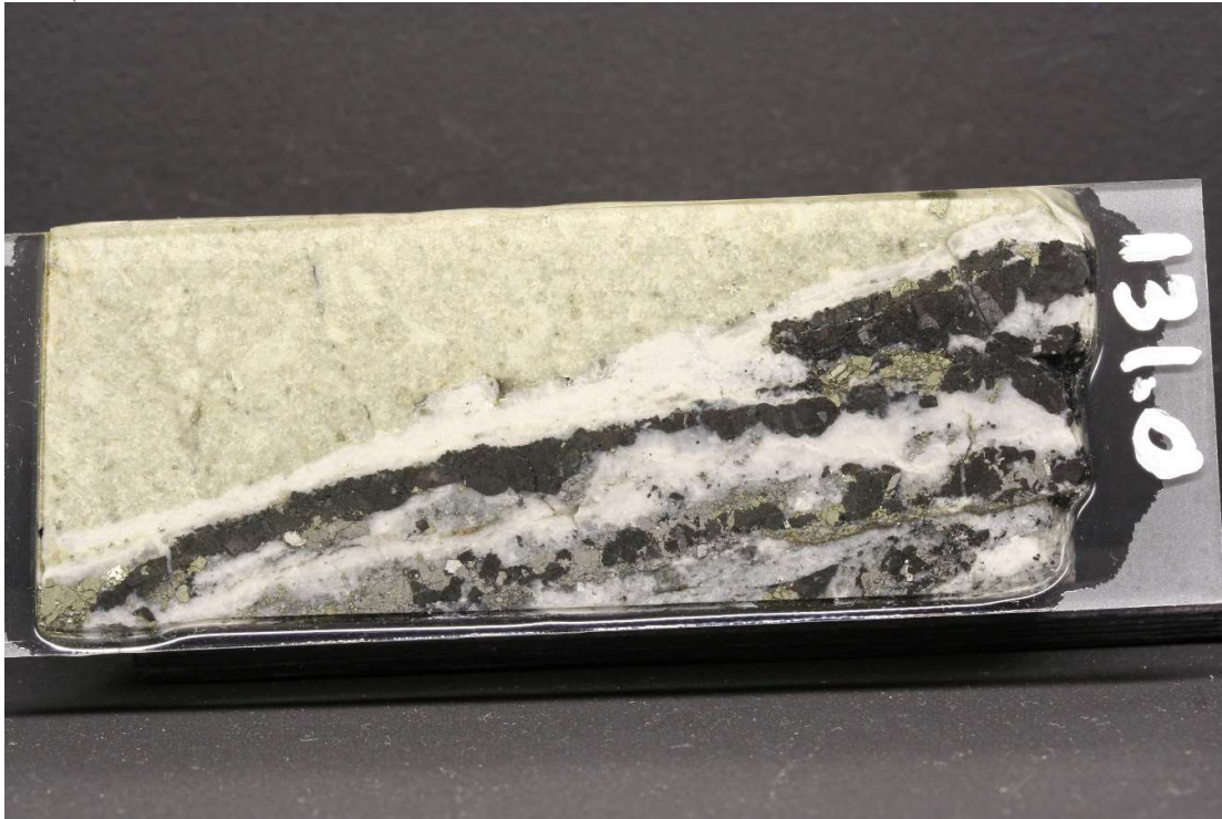
Fig 10. Mt Cannindah Mineralization Style Late sulphidic gold bearing vein QMCMDD007, 131.00m. sericitised felsic porphyry with gold-bearing sphalerite-arsenopyrite-pyrite-ankerite vein. Qld Ores core photo – 2008 report.
