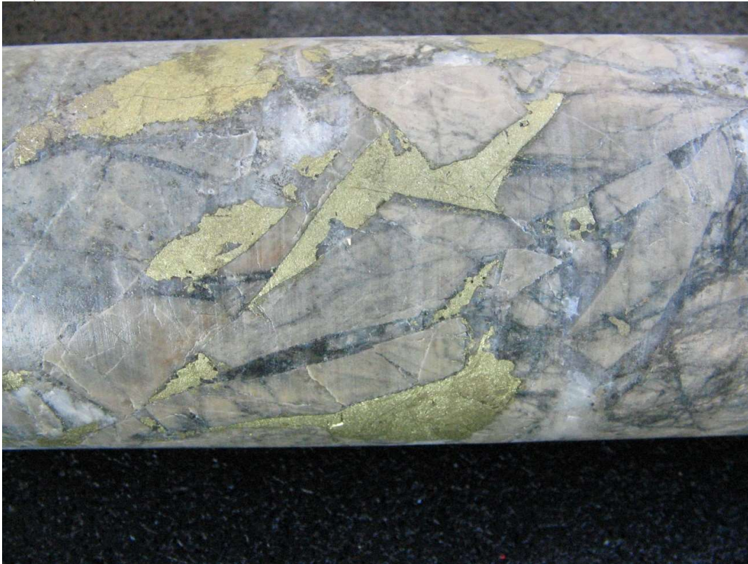
Fig 4. Mt Cannindah Mineralization Style : Breccia Infill in metasediments: QMCMDD022, 260.00m. Infill Breccia, chalcopyrite-pyrite. Qld Ores core photo – 2008 report.
