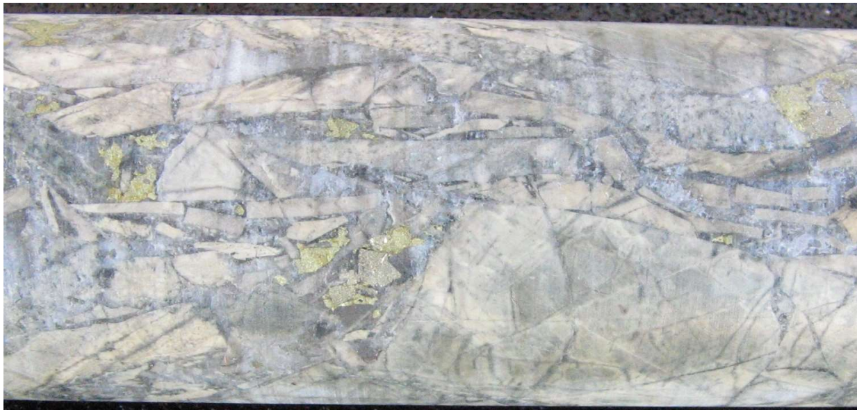
Fig 5. Mt Cannindah Mineralization Style : Breccia Infill in metasediments.(QMCMDD022). 'Splinter' breccia. The 'splinter' breccia was probably produced by fluid pressure cracking an overpressurised carapace. Dilational structures have acted as conduits for ore fluids from a potential stock at depth. Qld Ores core photo – 2008 report.
