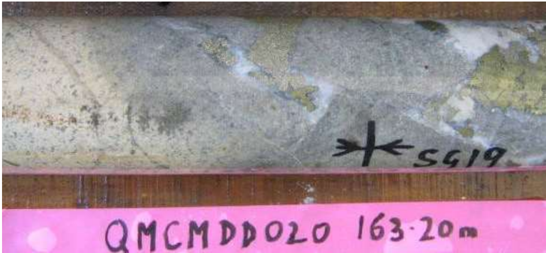
Fig 8. Mt Cannindah Mineralization Style Intrusive hosted Vein & infill. QMCMD020, 163.20m, Brecciation and infill chalcopyrite pyrite mineralisation initiating via opening of joint sets. Qld Ores core photo – 2008 report.
