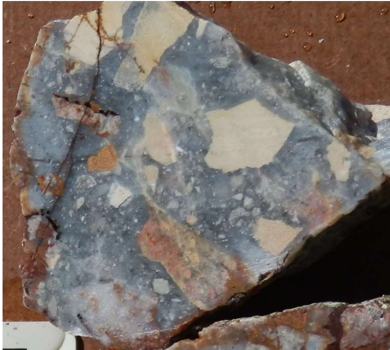
Fig 11. BAR033.Sulphidic polymict breccia, clasts sandstone and porphyry , silica –marcasite matrix. . 204 ppm As, 80ppb Au.
