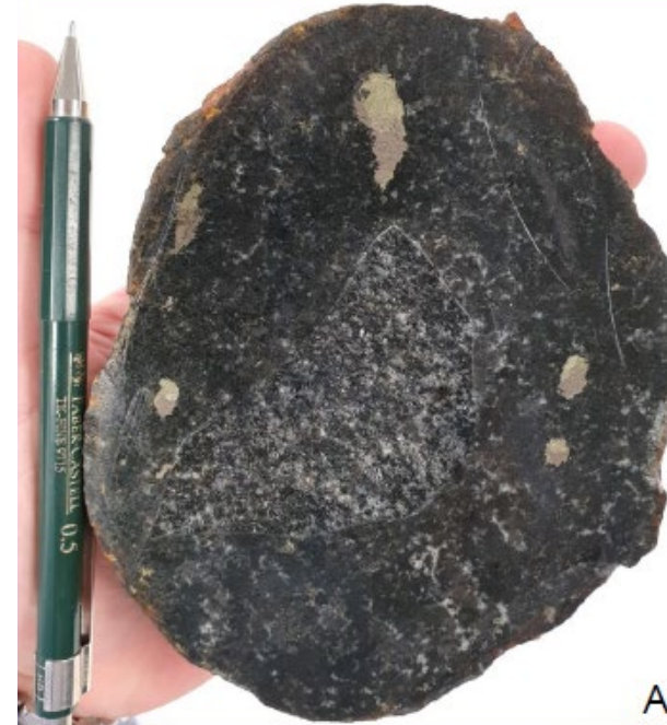
Coarse grained mafic intrusion showing high tenor three phase disseminated and blebby sulphides comprised of chalcopyrite, pentlandite and pyrrhotite
