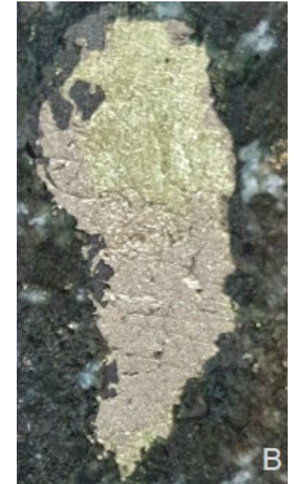
Coarse grained mafic intrusion showing high tenor three phase disseminated and blebby sulphides comprised of chalcopyrite, pentlandite and pyrrhotite
