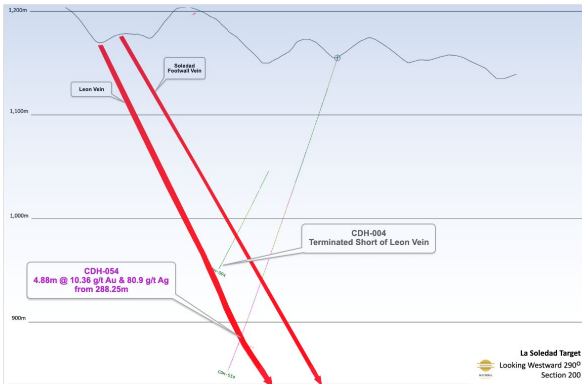
Figure 4 Cross Section 200 at La Soledad target showing hole CDH-054 and hole CDH-004 which terminated short of the Leon vein. Hole CDH-004 to be re-entered and drilled further 40m.
