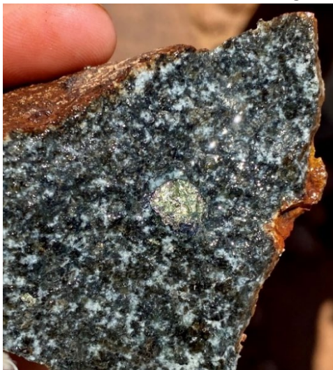
Figure 3: GLRK008A showing a three-phase blebby sulphide with chalcopyrite, pentlandite and pyrrhotite within a Gabbro.
