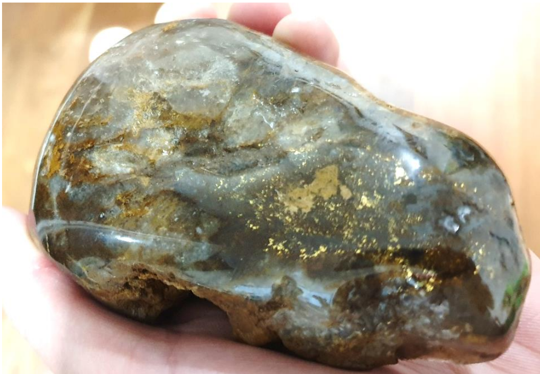
Figure 1: Photograph of recently polished gossanous quartz vein with abundant visible gold recently sampled by Silver City from the outcrop exposures in the north face of the Brians historic pit.
