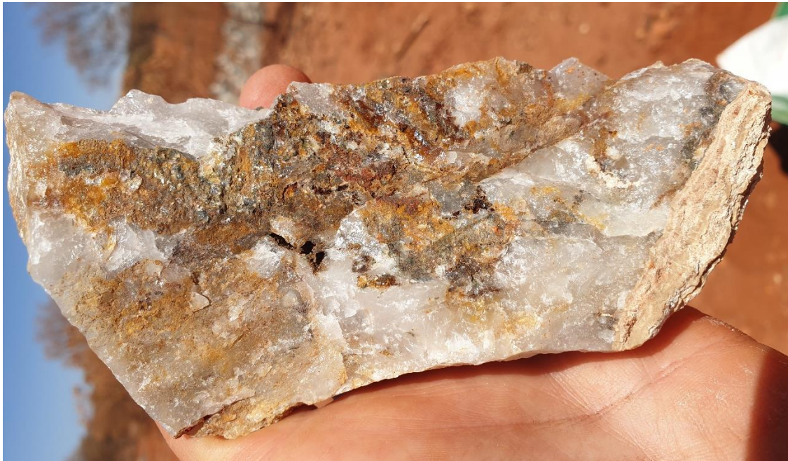
Figure 3: Example one of the weathered, gossanous quartz samples from ARK025 that returned high grade gold assays. Note the white/cream calcrete section to the right.
