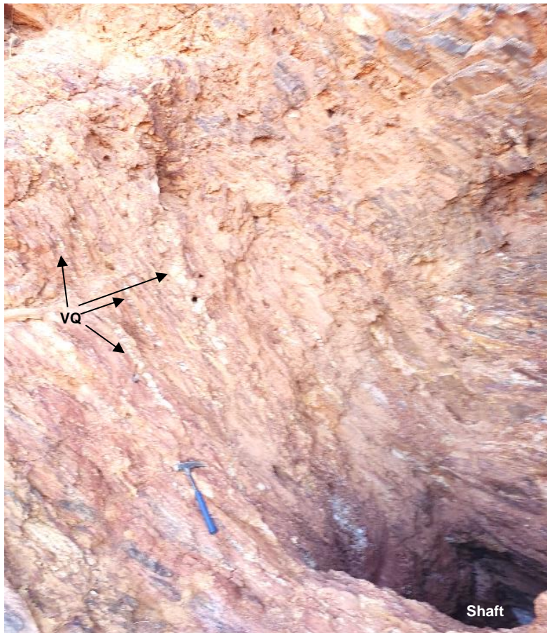
Figure 4: Mt Sandy adit showing multiple narrow quartz veins (VQ) where ARK020 was sampled.
