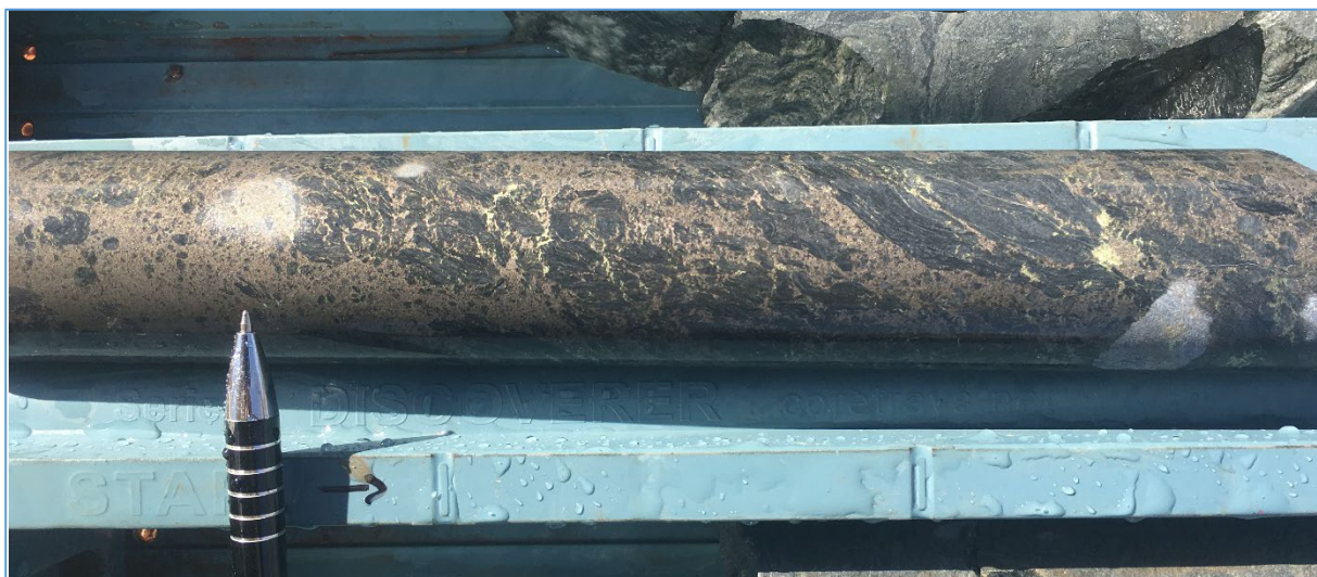
Figure 3: Diamond core from hole 20WD001 at 552.3m showing semi-massive pyrrhotite (bronze colour) and chalcopyrite (yellow) mineralisation.
