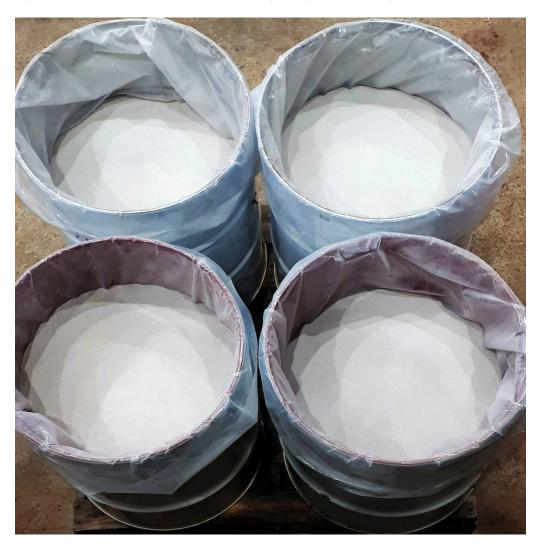
Sub samples were taken from the screened bulk sample and these samples have been used for spiral processing release testwork. A new MG12 spiral silica test rig was prepared by MT for these processing tests. Test fractions were weighed and split samples were assayed.
