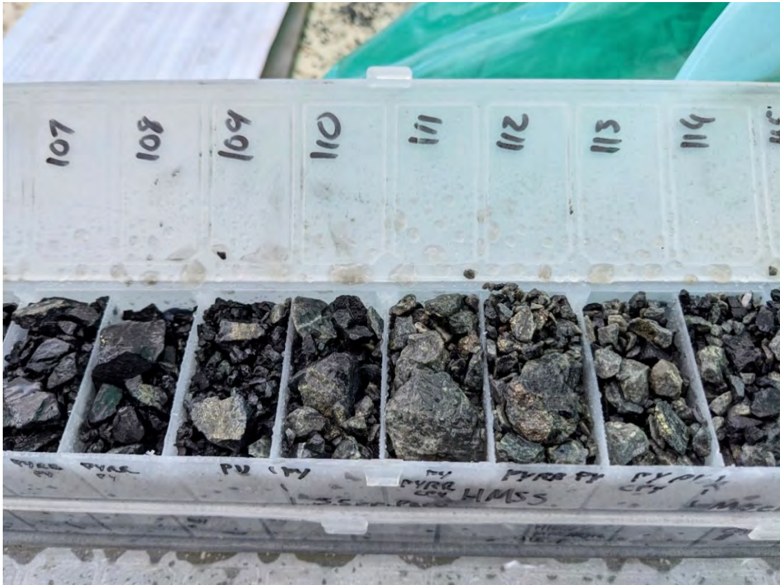
Figure 7. Drill chips of chalcopyrite from massive sulphide veins intersected by the VTEM anomaly drilling at Mt Flora.
