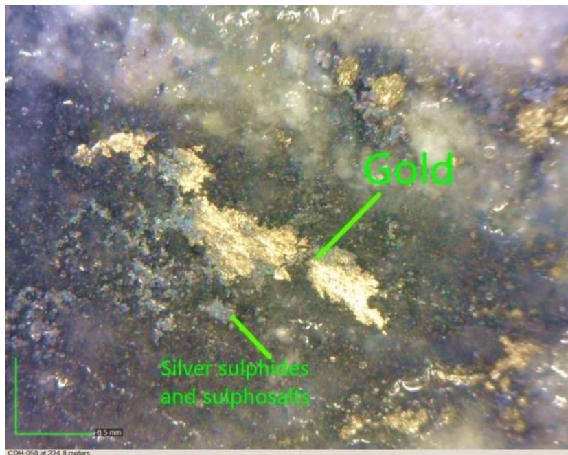
Figure 5: Visible gold and silver minerals in El Refugio drill core from CDH-050 at 234.8m
