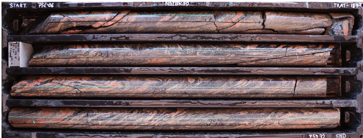
Photo 3. NDIBK10 (756.06 – 759.32): Equicrystalline qtz-plg-kfp-bio-mus granodiorite with poorly-developed schistose texture expressed mostly by bio and mus. Hem-altered 2 cm chilled margin (only slightly finer-grained than rest of unit) on lower boundary. No chilled margin or alteration at upper margin. Biotite partially weathered to hematite, particularly near upper and lower contacts. Minerals present (quartz, plagioclase, k-feldspar, biotite, muscovite).
