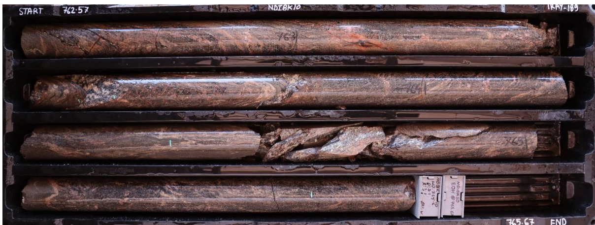
Photo 4. NDIBK10 (762.57 – 765.67): Qtz-biotite-amphibole schist of psammitic protolith and minor granitoid protolith (kfp regions). Cut by qtz-kfp-muscovite pegmatites. All poly-deformed and gneissose in part. Minerals present (quartz, biotite, amphibole, k-feldspar, muscovite, hematite).
