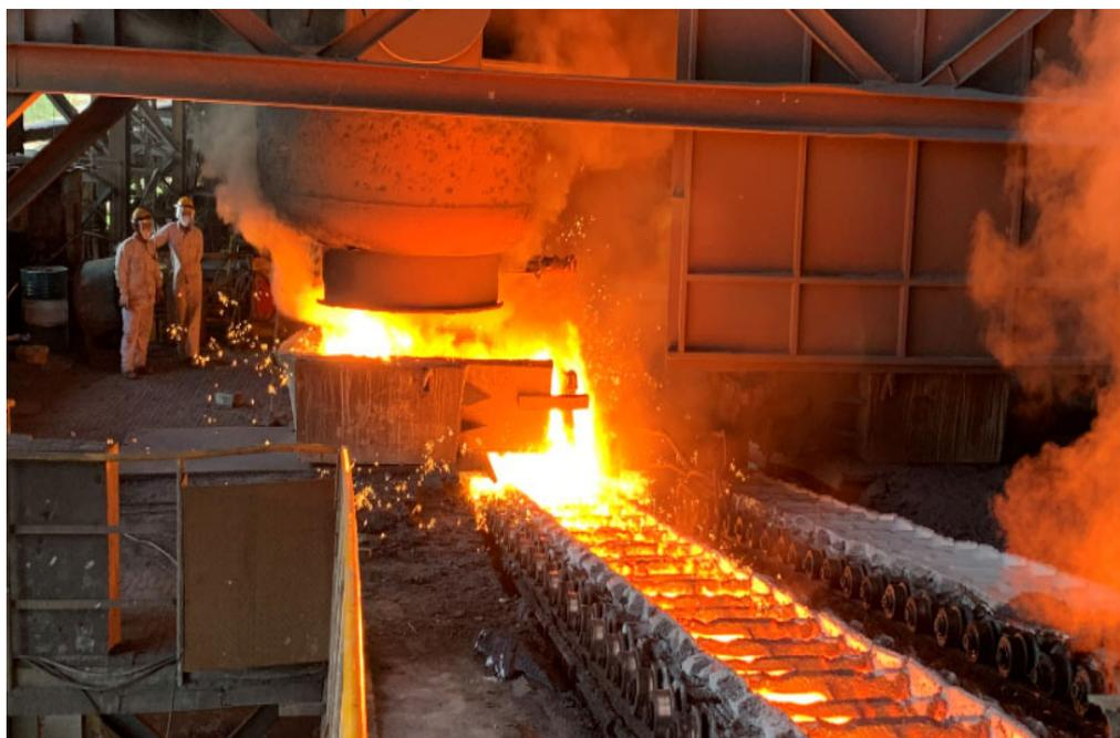
*Ingot casting of NPI*
