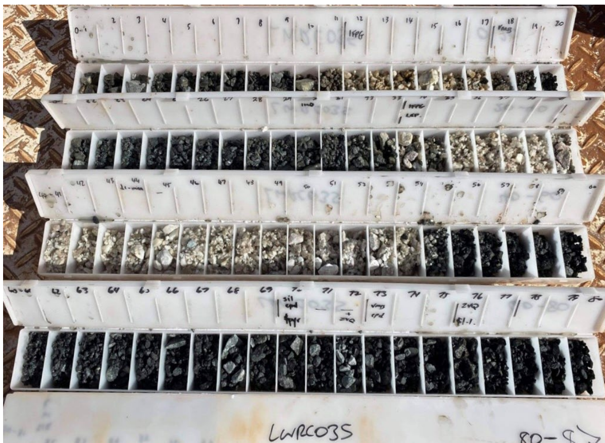
Figure 2: Image of the LWRC035 chip tray showing potentially lithium bearing pegmatite from 33m – 54m.
