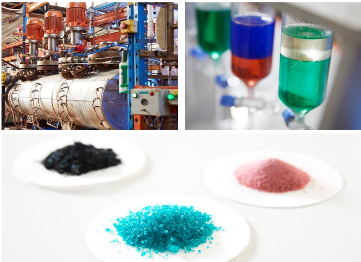
Figure 6: Collage of photographs taken of Australian Mines' demonstration scale processing plant in Western Australia, including images of the final cobalt sulphate (pink) and nickel sulphate (blue/green) and the intermediate mixed sulphide precipitate (MSP; black), which are routinely being produced.
