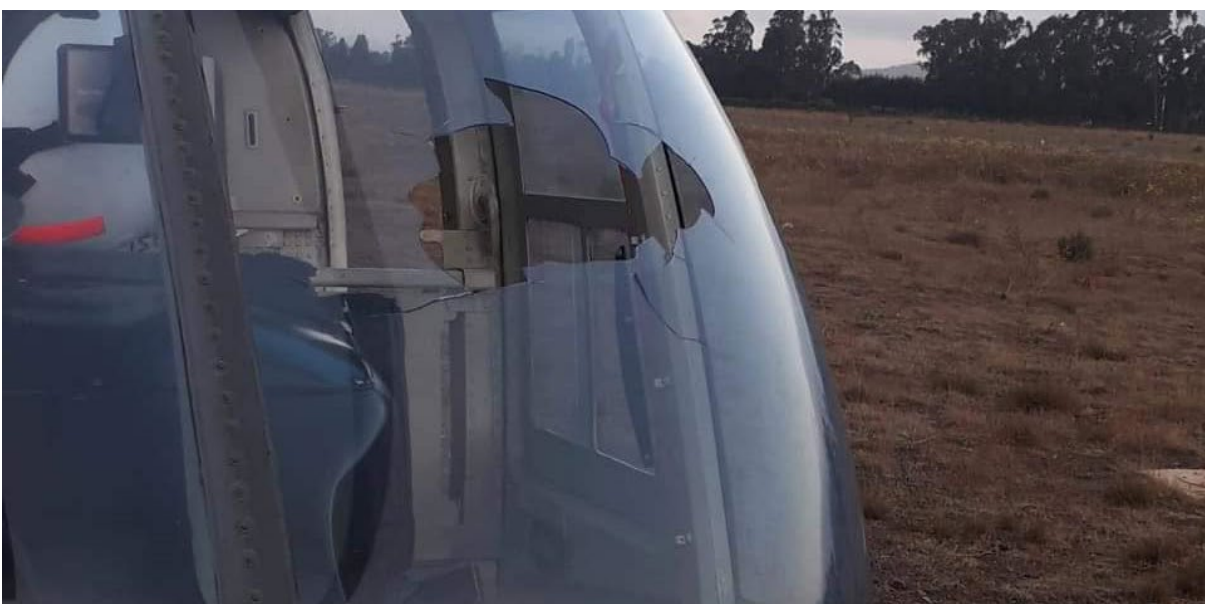
Image: Extensive damage to a Chilean Navy helicopter, which struck a drone causing significant injuries to a crewmember
