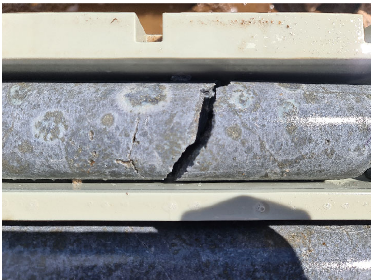
Plate 2 Mount Mackenzie South West slopes Primary High Sulphidation Epithermal Mineralisation
