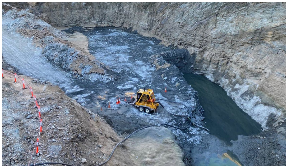
Plate 1 Granny Venn Pit Floor exposure at RL 380m following dewatering.
