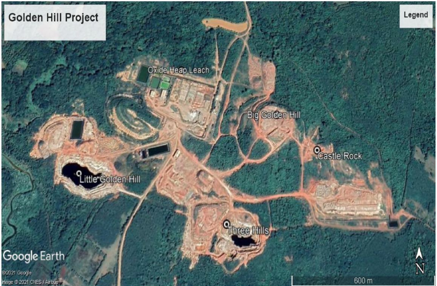
Mined oxide deposits at Golden Hills underlaid by an outcropping interconnected sulphide deposit
