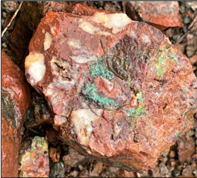
Figure 1. Malachite (green \text{Cu}_2\text{CO}_3(\text{OH})_2 ) contained within quartz breccia and jasper (red) from the Fairlight prospect. The copper-rich rocks occur along the contact between jaspers and metamorphosed mafic rocks of the Chillagoe Formation.
