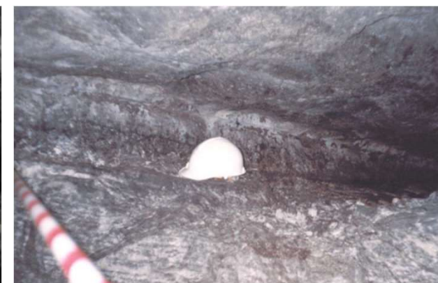
Mining at a height of sub 0.6 m - designed for operating in narrow-reefs
