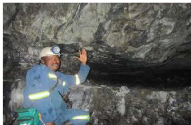
Mining at a height of sub 0.6 m - designed for operating in narrow-reefs
