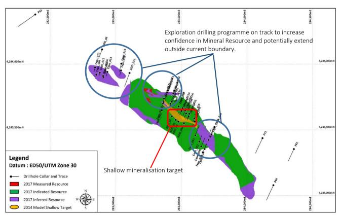
Figure 2. Oropesa geological resource depicting the diamond drilling program and proposed diamond drill hole locations.
