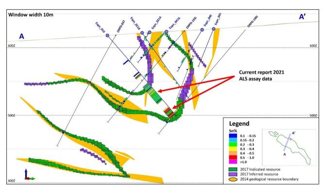
Figure 4. Oropesa 2021 resource infill diamond drilling, Expn\_016.
