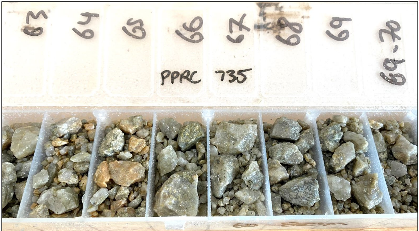
Figure 3: Photograph of chip tray from PPRC735 containing assay of 1m @ 96g/t silver from 66m, displaying strong sericite and silica alteration.
