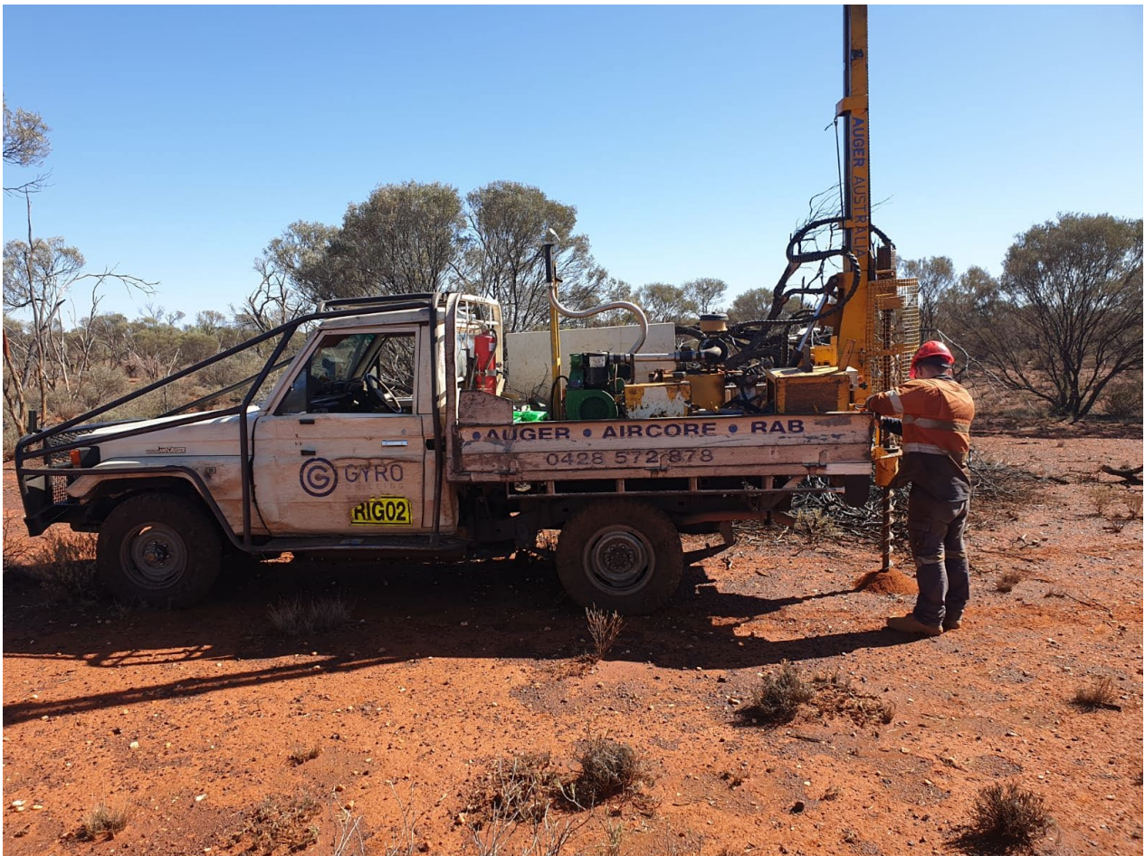
Figure 1: Gyro Australia’s Landcruiser mounted auger drilling rig will be used to maintain low impact disturbance and collect geochemical samples. Picture from Gyro Australia’s library.
