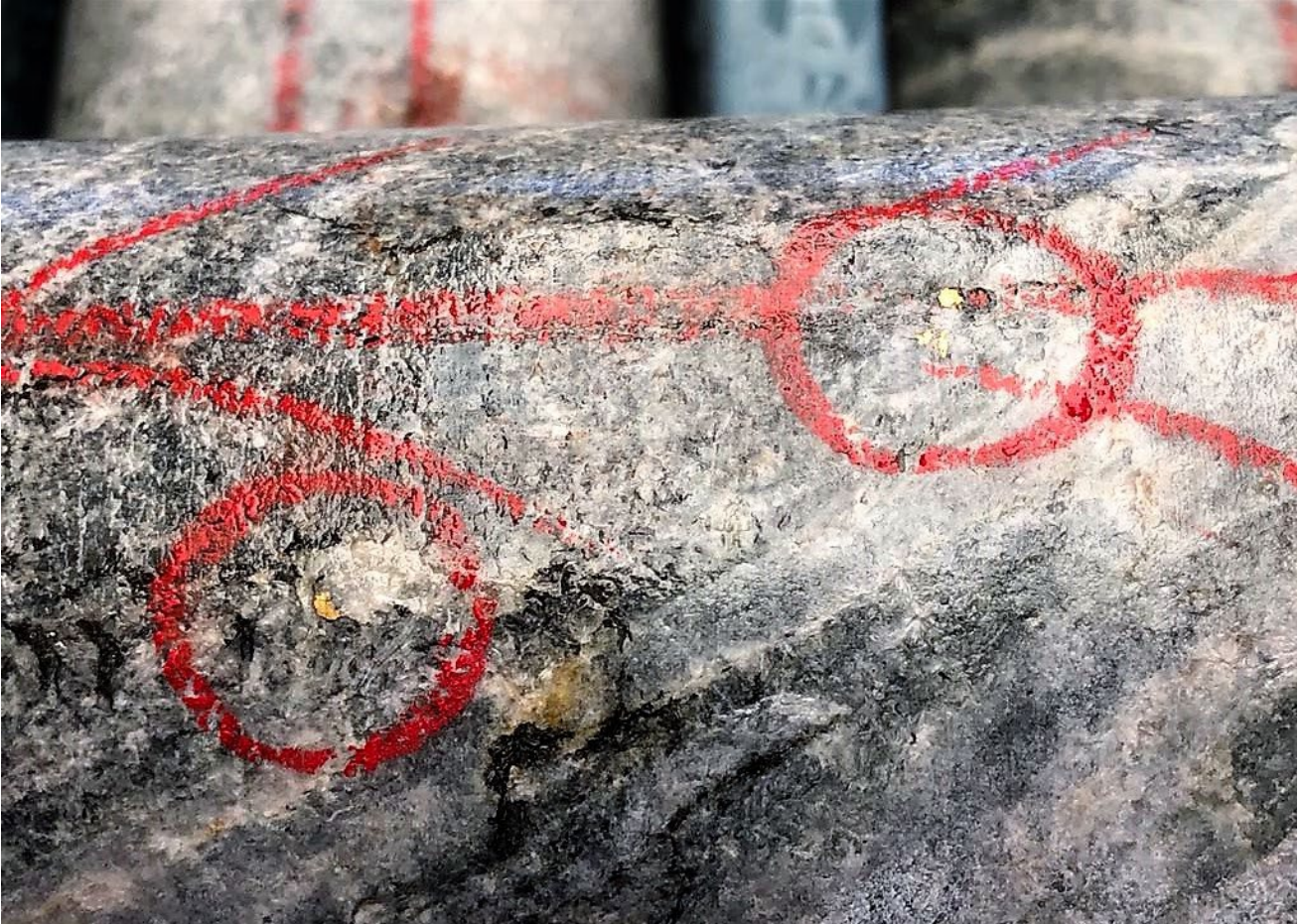
Figure 3. HQ Drill hole S05DD003 with visible gold at 80m depth. Visible gold does not characterise all mineralised intercepts at the S5 prospect. Red chinagraph lines are approximately 4mm wide, for scale.
