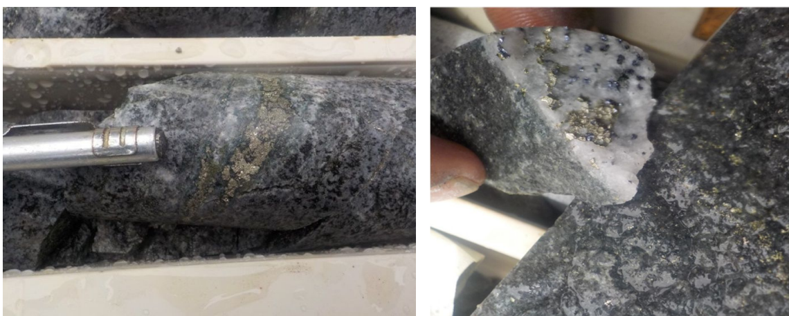
Figure 4. Micro-diorite (577.0m) showing qtz-pyrite-chlorite vein (LHS) and quartz – pyrite-Moly vein (RHS) at 437.40m
