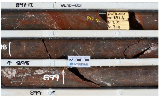
WLTD001, 897-899m, Murdie Project: IOCG-style hematite alteration and brecciation.
