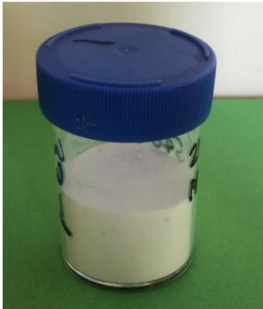
Above: Alcore  $\text{AlF}_3$  sample produced from a combination of dross and aluminium hydroxide.
