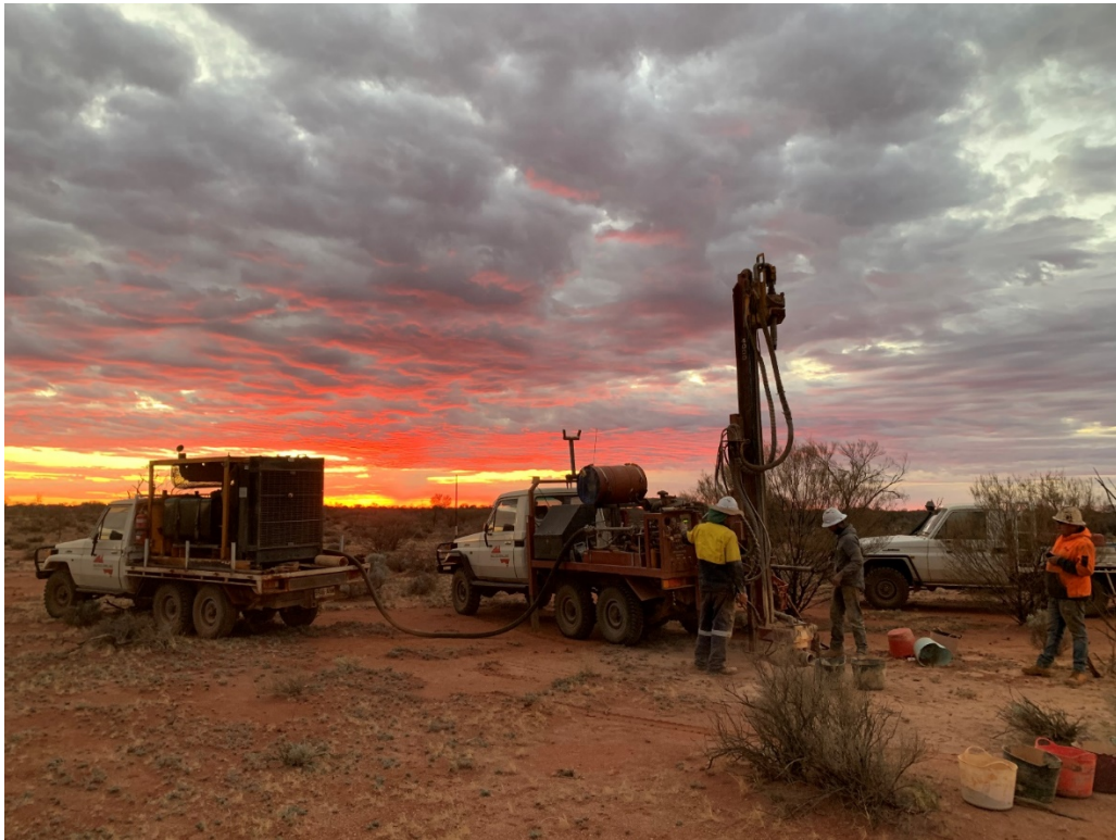
Shallow RAB Drilling Operations at Comet (May 2021)
