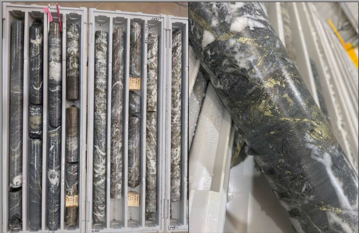
Figure 1 – Semi-massive pyrite-pyrrhotite-chalcopyrite and quartz-pyrite-pyrrhotite-chalcopyrite breccia approx. 184-193m downhole in IDD001 .
