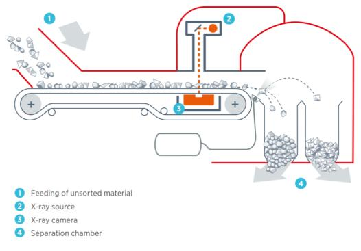
Figure 3: Tomra<sup>™</sup> ore sorting schematic
