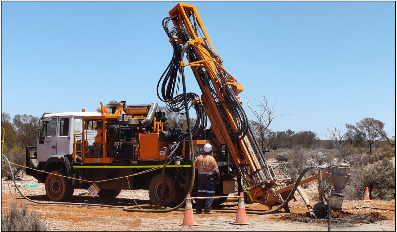
Figure 1 - Rainbow Dam RC drilling - Photo courtesy of Salazar
