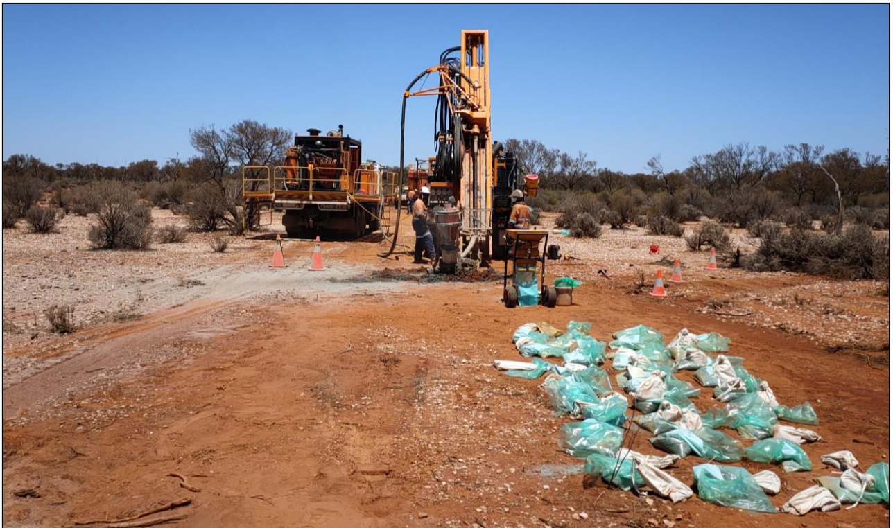
Figure 2 – Samples ready of collection at Rainbow Dam RC drilling - Photo courtesy of Salazar
