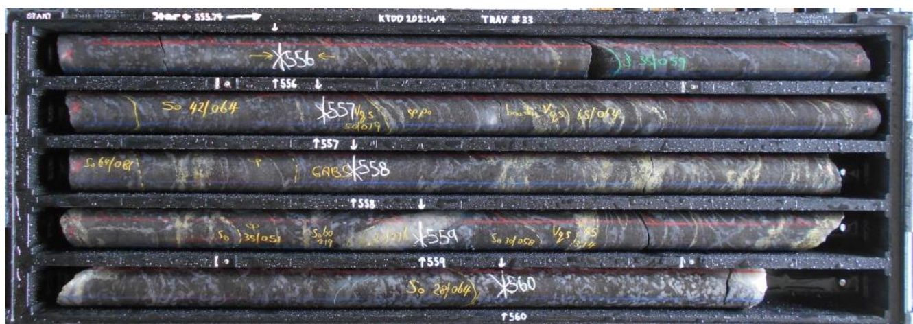
Figure 3 Cu-Au mineralisation in KTDD202_W4 in Kavanagh from 555.74m to 560.32m The interval 557 to 560m is an average of 3m @ 2.23% Cu, 0.19 g/t Au.
