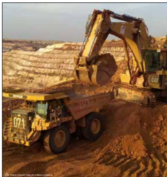
Figure 28: Tubani Pit fresh pit cut-back stripping oxide zone, Kintinian Mine area. Refer Figure 27 for location. These pictures give a feel for the extensive scale of the AGA operation related to the low grade of mineralisation and nature of the oxide (brown) and saprolite zones (pale/whitish).
