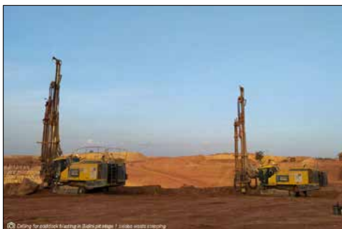
Figure 29: Bidini Pit Stage 1 Oxide waste stripping, drilling paddock for blasting in AGA Kintinian Mine area. Refer Figure 27 for location.
