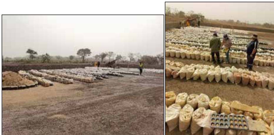
Figure 48: GGR/Polymetals sample storage yard with bulk RC drill cuttings in Alahiné Village field exploration compound. Samples are weighed and split for dried samples and as required for sample dispatch to the assay laboratory. Detailed logging of cuttings is undertaken at this site and chip boards made for reference at this early stage of the program which has aided offsite assessment of drill sections due to travel restrictions.
