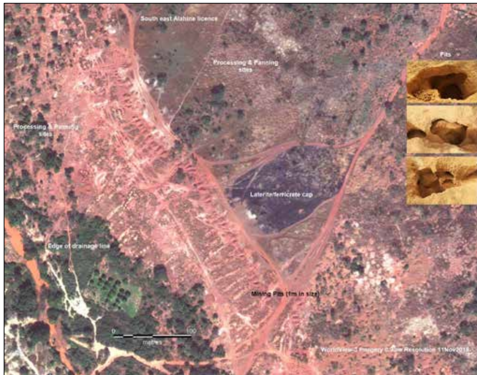
Figure 38: Detail from Figure 37 showing extensive surface workings along trend of major north north-west drainage line. This may be reflecting structural deformation in the basement rocks through the licence which is an important requirement for the presence of veins which host gold mineralisation. Figure 37 shows the extension of this zone northward. Photographs of 3 pits are shown as insets on the right. (Zoom in to see in more detail).
