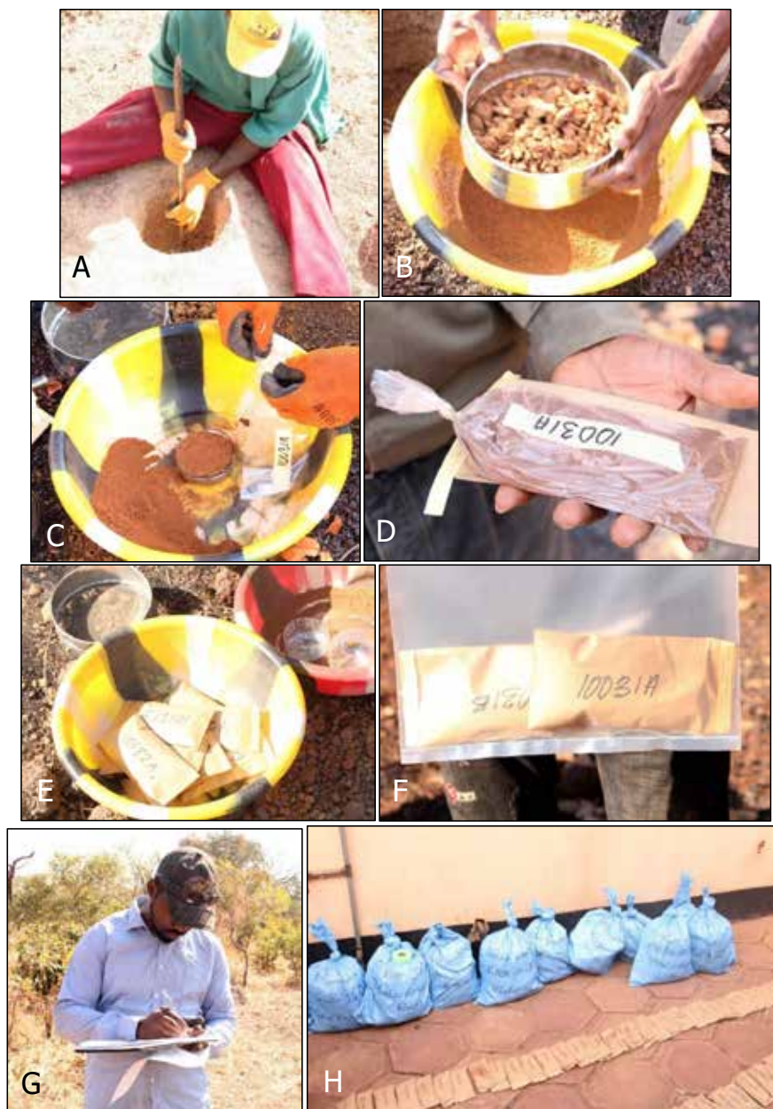
Figure 67: Field Sampling (A) Sampling hole 30-60cm deep; (B) Sieving -2mm fraction; (C) Placing sample in plastic bag; (D) Double bagging with outer kraft paper to avoid spilling and cross contamination; (E) Sampling equipment; (F) Composite pairs labelled "XXX"A & "XXX"B bagged together; (G) Geologist logging hole at sample site; (H) Samples sorted and bagged for transport to laboratory (Golden Guinea local company licence holder owned by Polymetals).
