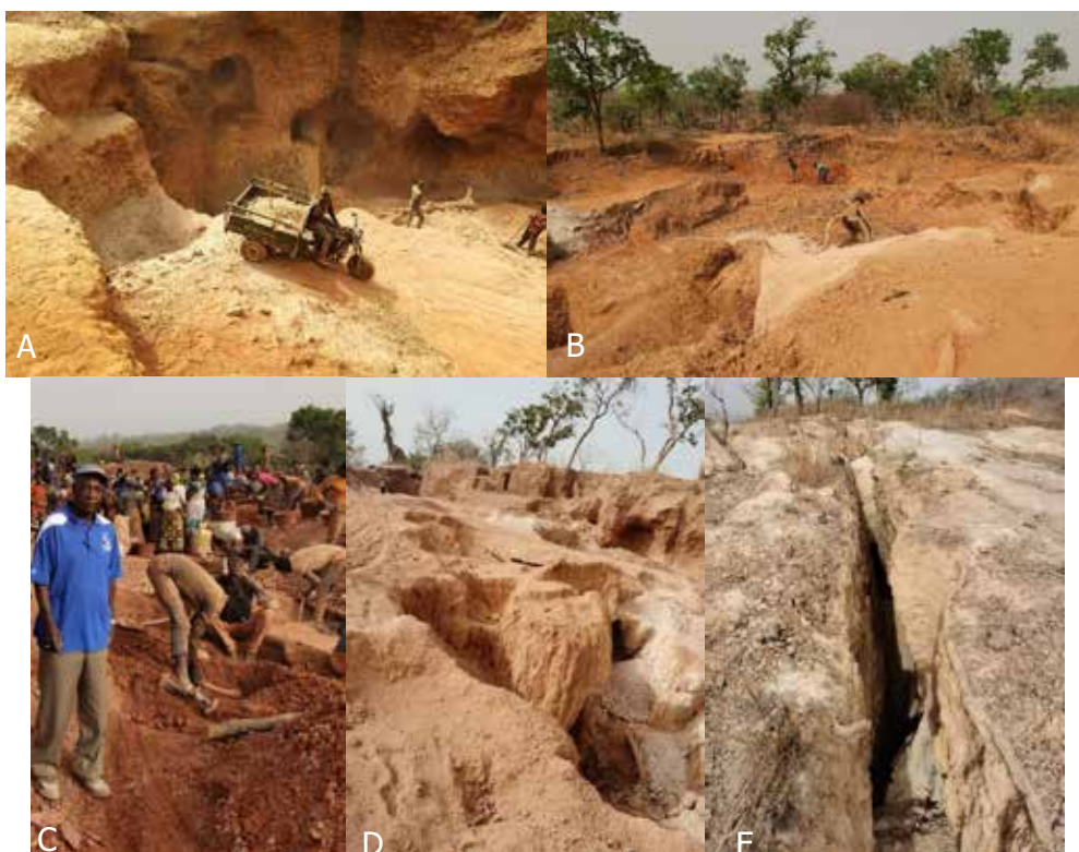
Figure 35: Examples of artisanal mining activity in Alahiné licence. A: Mining basal colluvial ferricrete contact zone over saprolite; B: As for A, "palaeoalluvial" sites; C: Active artisanal diggings and processing; D and E: Pitting on narrow veins in saprolite at ferricrete cap contact with basement saprolite and in window of basement exposure.
