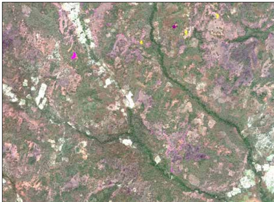
Figure 63: Central and eastern section of Mansala licence showing drainage lines cutting through laterite surfaces (purplish shaded patches). (Refer Figure 49 for scale).
