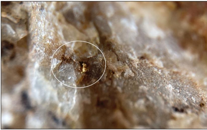
Figure 4. One of many grab samples found containing visible gold. The gold here, which is less than 0.5mm, is associated with a small fracture in the quartz containing oxidized material. This small piece of gold has a different habit to the flakes found in white quartz. No samples containing visible gold were used for assay.
