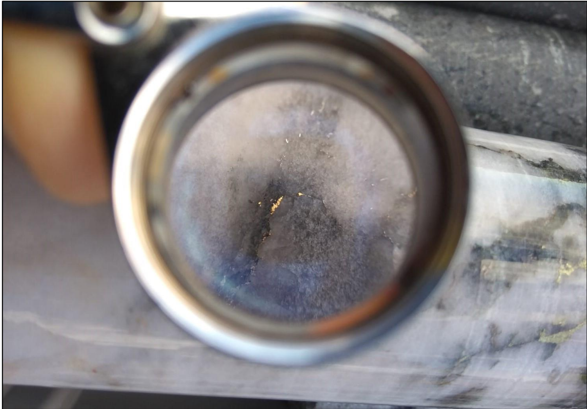
Figure (1): Visible gold observed in diamond drill core from hole GDD018, correlating to an interval of 1.9 metres @ 22.4g/t Au from 151.4m. Note hand lens 10x magnification.
