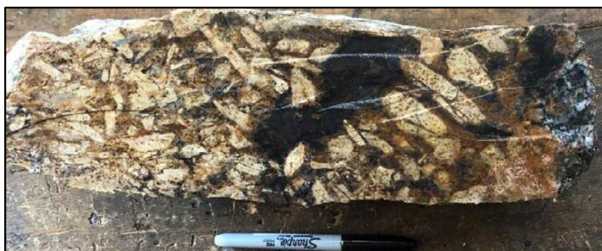
Photo 4: McCrossin's Prospect - brecciated volcanics with disseminated sulphides and gold mineralisation
