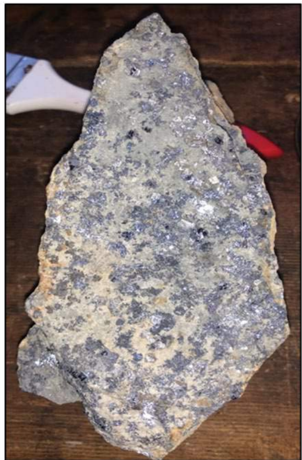
Photo 1: Silver bearing galena mineralisation from Webbs Consol's main shaft
