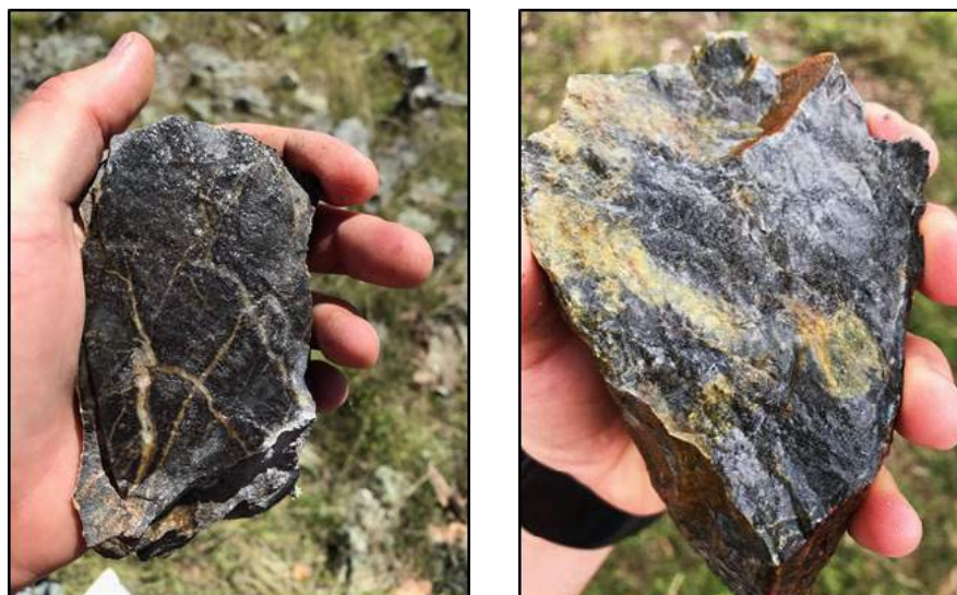
Photo 2: Hudson's Prospect – Stockwork quartz veining and disseminated arsenopyrite in silicified siltstone hosting gold mineralisation
