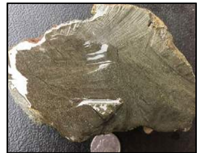
Photo 6: Trough Gully Mine – banded sulphide veining
