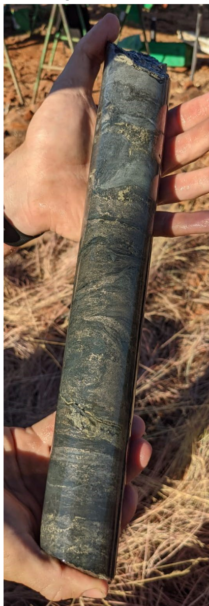
Figure 1: Pyrrhotite and minor pyrite and chalcopyrite in Ruins Dolerite at 56.75m from TXDD001.
