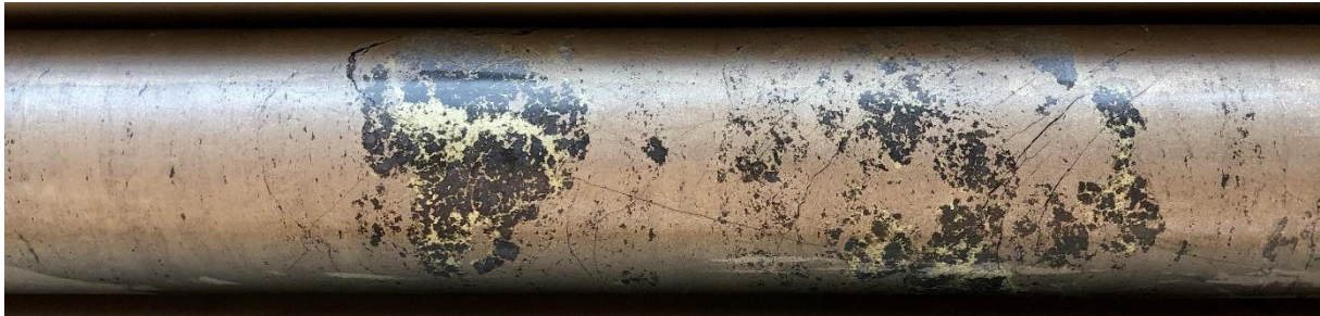
Figure 2: Diamond core of massive sulphide drilled at Chianti in 2019 (CHDD002 116.4-120m @ 1.0% Cu, 4.9g/t Ag).
