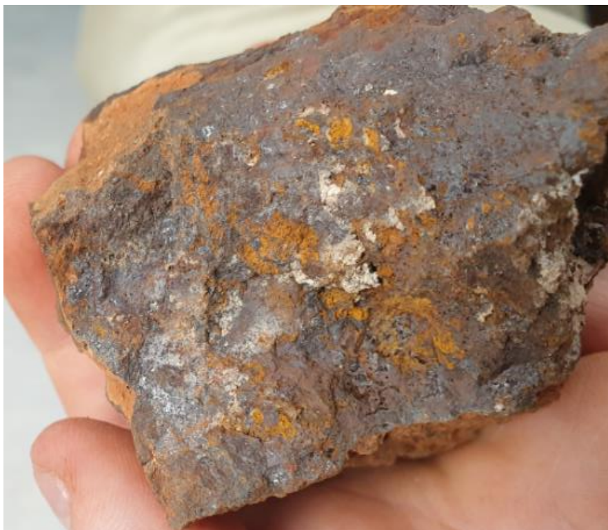
Figure 1: Rock chip sample MNRK0366 showing limonitic staining around boxworks (0.4% Cu, 0.4% Ni, 0.03% Co, 0.3 g/t Pt-Pd-Au).
