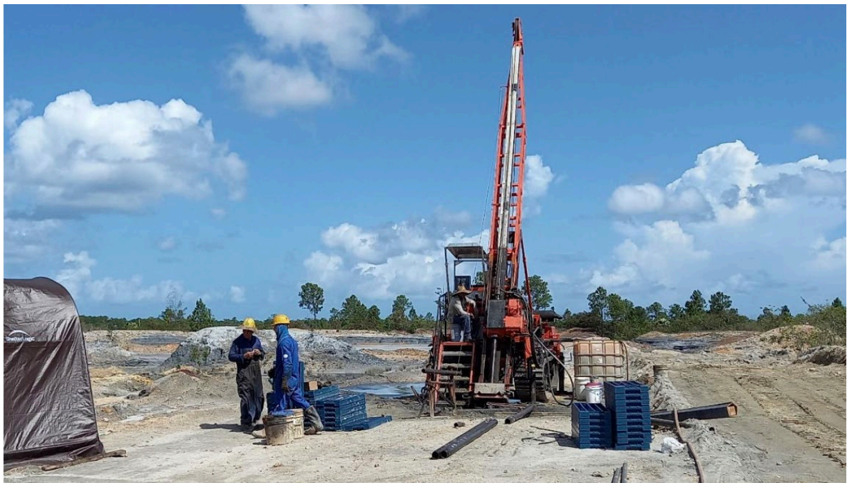
Larger drill rig recently engaged for +200m cored holes.
