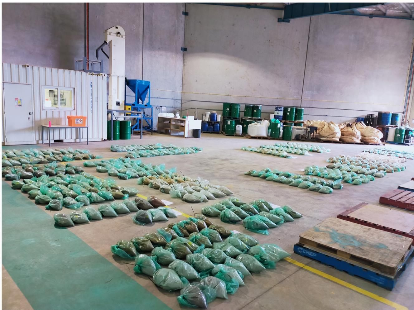
Figure 9: Preparation for Metallurgical testing of Cape Flattery Silica Sand
